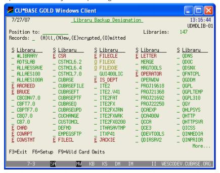
The system first performs a scan (UDMDLIBCL) for any new libraries that have been added since the last time the configuration was done. The screen shows all libraries on the iSeries and any existing encryption codes you have set up.
